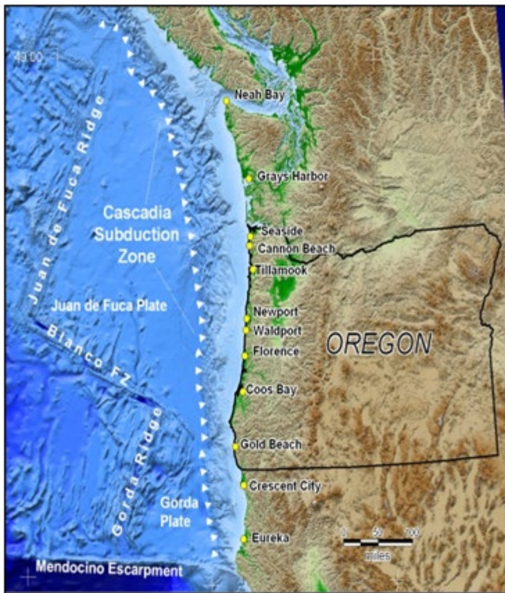
Figure 3.3.8-2: Cascadia Subduction Zone (CSZ) Active Fault Map. The fault, indicated by the triangles, is the contact where the Juan de Fuca Plate plunges beneath the North American continental plate.
