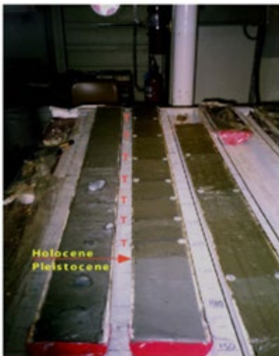
Figure 3.3.3-3: Deep Sea Sediment Cores that Record Past Megathrust Earthquakes off the Oregon Coast
