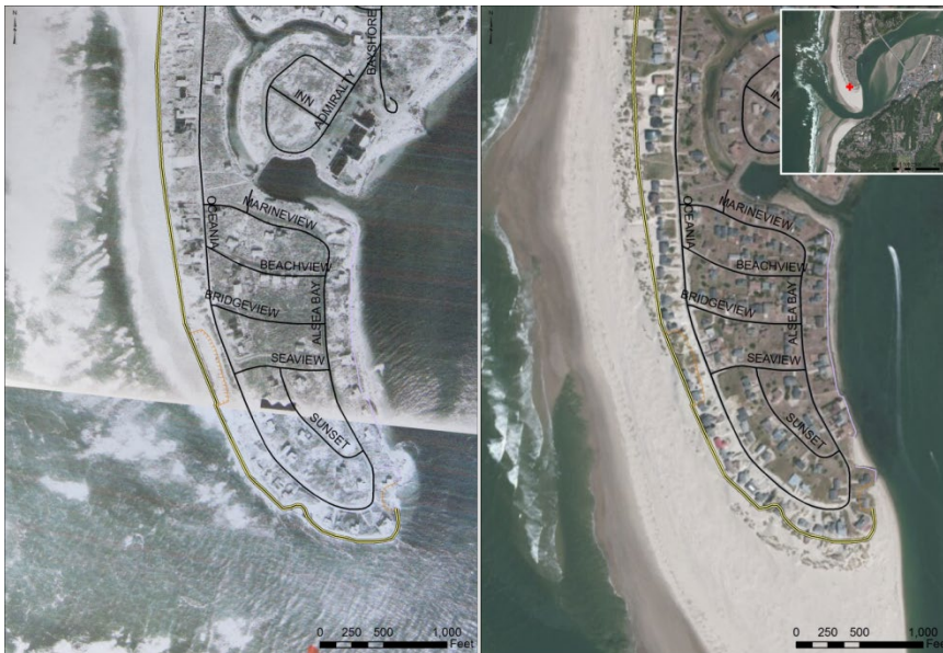
Figure 3.3.1-8: Alsea Bay Spit Erosion as a Result of the 1982-83 El Niño (left), and State of the Beach in 2009 (right)
