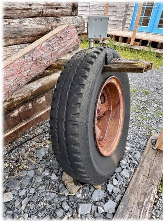
Figure 9: Impaled Tire, Whittier, Alaska. Photo by OEM, 2025. The tire was impaled by the piece of 2X12 lumber during the March 1964, M9.2 subduction zone earthquake .
