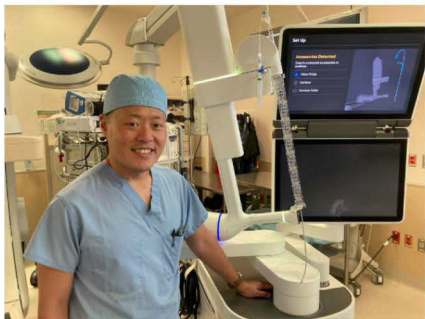
OHSU interventional pulmonologist Peter Lee, M.D., M.H.S., helps people with lung nodules using the Ion robotic navigation system (nicknamed Rosie). Under Lee's direction, the system guides a thin probe through a patient's lung to examine nodules for signs of cancer. He is one of the medical co-directors of OHSU's new lung cancer screening program. (OHSU/Chris Lydgate)
