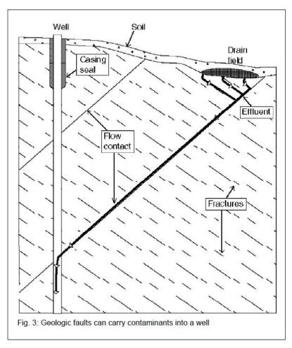
the effluent from the drain field to the well. Contaminants migrated along the inclined permeable contacts between individual flows to the well bore.
