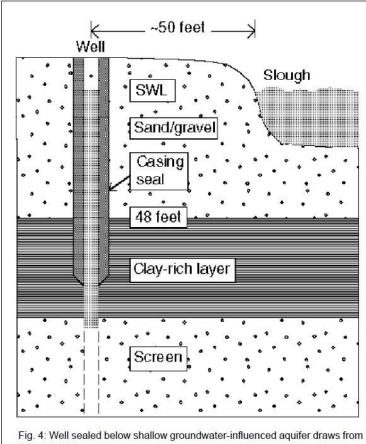
The fact that this well is not under the direct influence of surface water means the system will not have to install filtration. The upfront expense of installing a casing seal to 55 feet is minor when compared to the cost of installing and maintaining filtration treatment.
