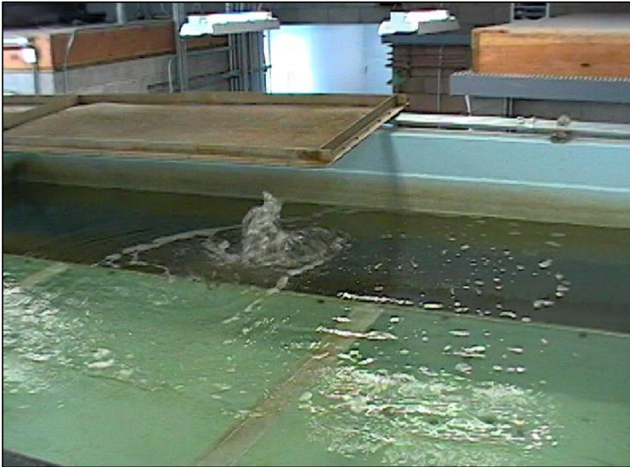
Air binding in a contact adsorption clarifier in California
