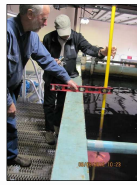
Measuring Filter Bed Expansion Ilwaco CPE 2012
