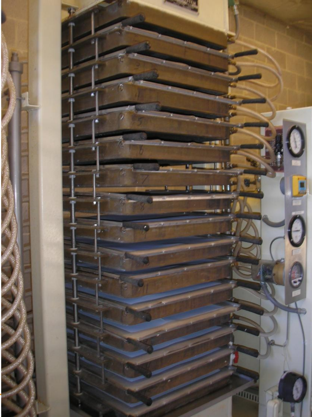
DE filter stack
