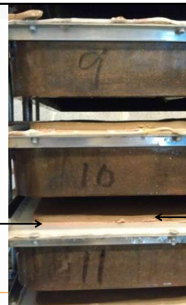
Sediment that's been filtered out (brown layer)
