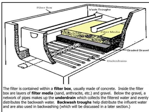
The filter is contained within a **filter box**, usually made of concrete. Inside the filter box are layers of **filter media** (sand, anthracite, etc.) and gravel. Below the gravel, a network of pipes makes up the **underdrain** which collects the filtered water and evenly distributes the backwash water. **Backwash troughs** help distribute the influent water and are also used in backwashing (which will be discussed in a later section.)
