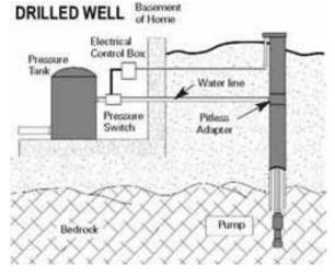
clay, should be poured along the outside of the casing to the top of the well. The well is capped to prevent surface water from entering the well.
