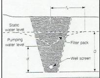
Figure 22.26. On-land infiltration gallery installed Figure 22.27. Terms used in the equation for determining the flow rate into the screen and the length of the screen
