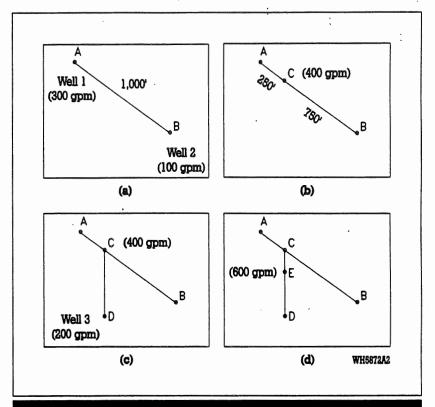
NOTE: Determination of location of single hypothetical well to replace actual wells in the case where individual CFR circles overlap. One circle is drawn with hypothetical well as center point having discharge equal to sum of all individual wells.
