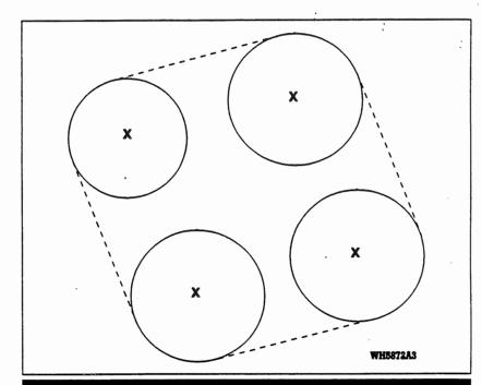
NOTE: Because of uncertainty associated with the calculated fixed radius method, a singleline (dashed in figure) is drawn to encompass all the individual circles. The area enclosed by the dashed line should be considered as the wellhead protection area for the wellfield.
