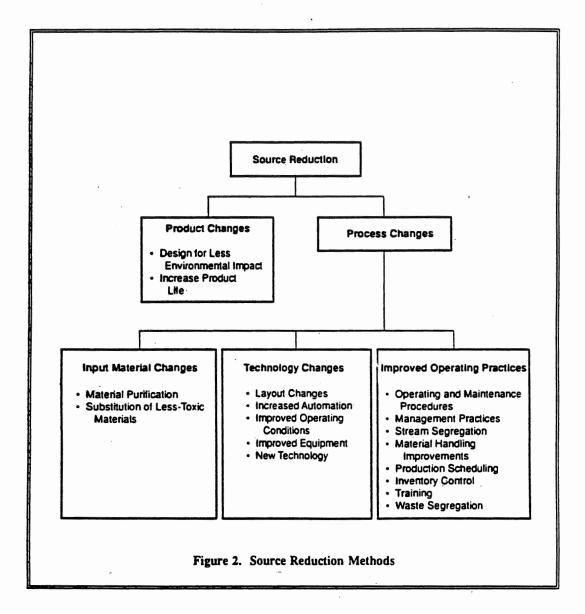
Process changes are concerned with how the product is made. They include input material changes, technology changes, and improved operating practices. All such changes reduce worker exposure to pollutants during the manufacturing process. Typically, improved operating practices can be implemented more quickly and at less expense than input material and technology changes. Box 2 provides examples of process changes.
