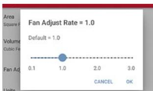
Touch Units to change pressure from Pascals to Inches of Water Column, or to change flow from CFM to metric units. (Inches of Water Column will put the DG-1000 in Pressure mode.)
