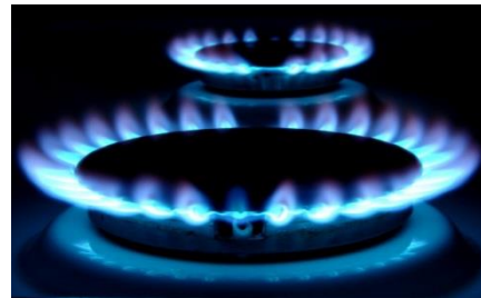
Uniform blue flames indicate a properly operating burner.
