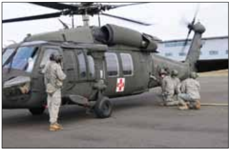
Soldiers of 2-641 Aviation, Oregon Army National Guard, Salem, Ore., conduct a “hot refueling” during Forward Arming and Refueling Point training at Army Aviation Support Facility 1, March 5. Hot refueling occurs at a stationary site, while only the pilots are left with the aircraft and the aircraft engines are reduced to an idle.
