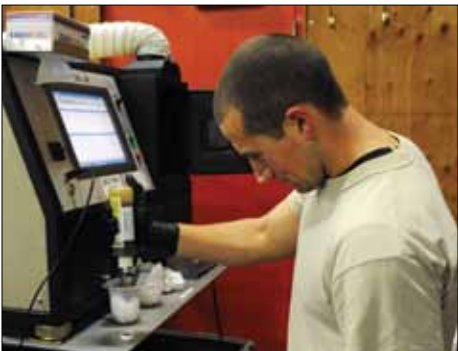
Staff Sgt. Christopher Campbell, 142nd Maintenance Squadron, performs jet engine oil sample testing during the unit's participation in Exercise Vigilant Shield 2017, Yellowknife, Northwest Territories, Oct. 19, 2016.
