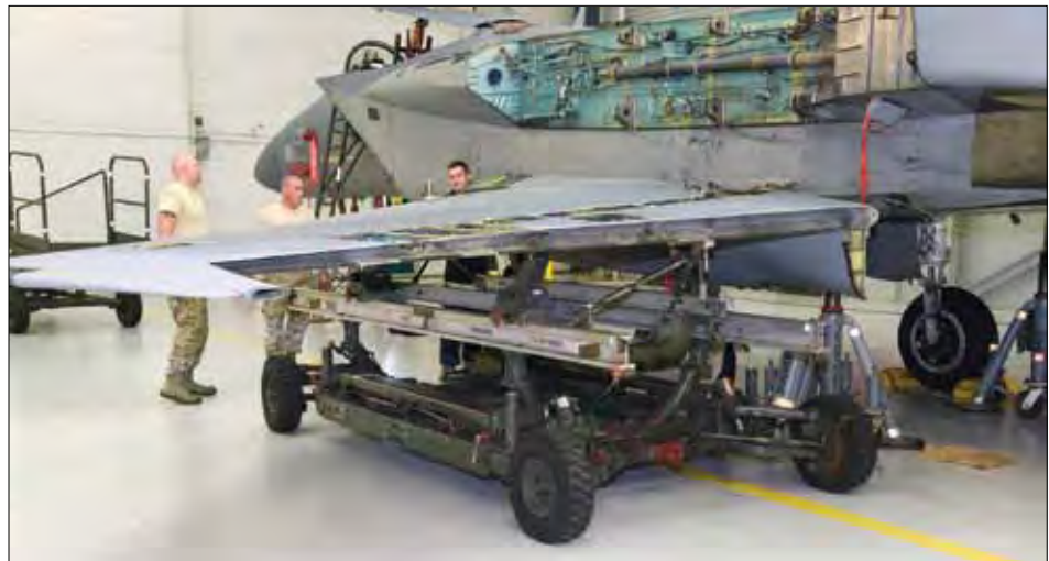
The Depot Field Team from the 402nd Aircraft Maintenance Group, Robins Air Force Base, Ga., remove the wing from an F-15C Eagle assigned to the 142nd Fighter Wing, Portland Air National Guard Base, Oregon, Dec. 6, 2016.
