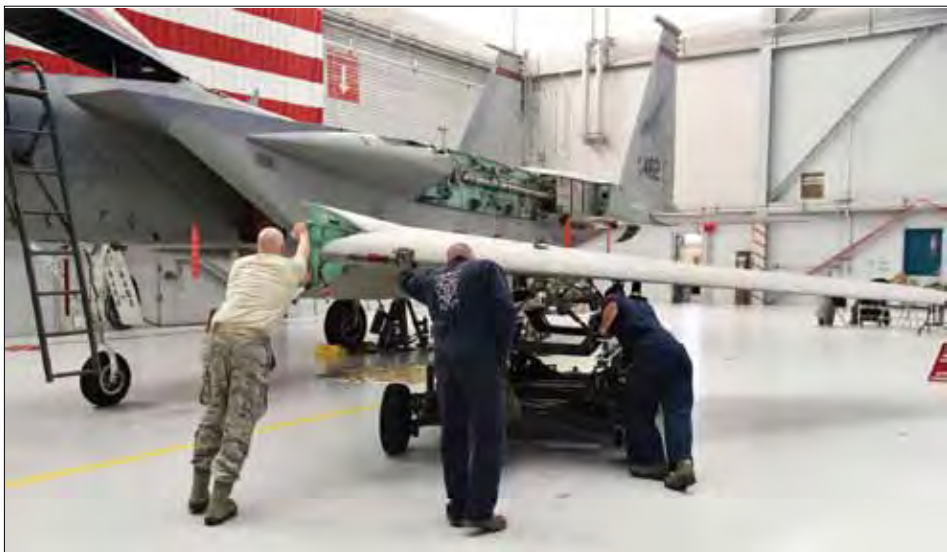
The Depot Field Team from the 402nd Aircraft Maintenance Group move the new wing into place during the wing replacement of F-15C Eagle 78-482, assigned to the 142nd Fighter Wing, Portland Air National Guard Base, Oregon, Dec. 6, 2016.
