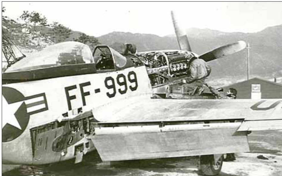
1st Lt. Ernie Wakehouse’s Mustang, FF-999, undergoes a 100-hour inspection by a maintenance team at K-46 Air Base, Korea, in 1951.
