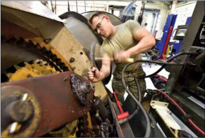
Tech. Sgt. Jacob Graham, a vehicle operations mechanic with the 173rd Fighter Wing, removes a cotter pin from a damaged plow roll-over assembly, Jan. 8, at Kingsley Field in Klamath Falls, Ore.
