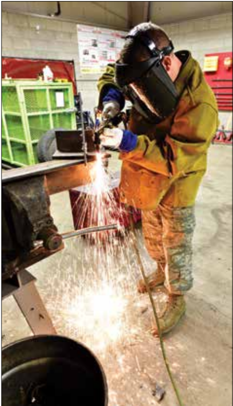
Master Sgt. James Childs, 173rd Fighter Wing vehicle maintenance shop, uses a cutting torch during fabrication of a support bracket for a roll-over snow plow, Jan. 14, 2019, at Kingsley Field in Klamath Falls.
