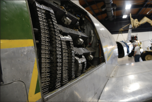
The weapons system on the F-86 Sabre is opened for inspection during the aircraft's final assembly.
