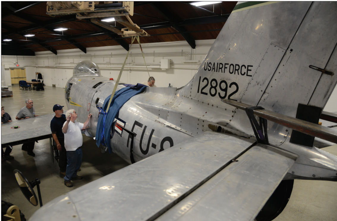
The two larger sections of the F-86 Sabre jet are brought together by a hoist and the aircraft is reassembled on February 26, 2020, at the Oregon Military Museum at Camp Withycombe, Clackamas, Oregon.
