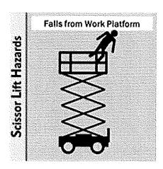
Scissor lifts must have guardrails installed to prevent workers from falling (see 29 CFR 1926.451(g) or 29 CFR 1910.29(b). [Note: for this section, the criteria and practices requirements for guardrail systems on scaffolds are contained in 29 CFR part 1926, Subpart L or 29 CFR 1915.73].
