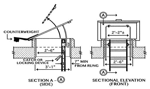
Individual-rung ladders are constructed to prevent the employee's feet from sliding off the ends of the rungs (see below);
