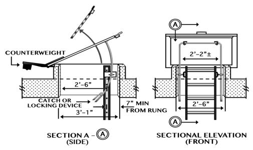
Individual-rung ladders are constructed to prevent the employee's feet from sliding off the ends of the rungs (see below);
