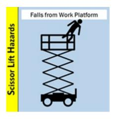
Scissor lifts must have guardrails installed to prevent workers from falling (29 CFR 1910.29b). [Note: for this section, the criteria and practices requirements for guardrail systems on scaffolds are contained in 29 CFR 1926, Subpart L or 29 CFR 1915.73].
