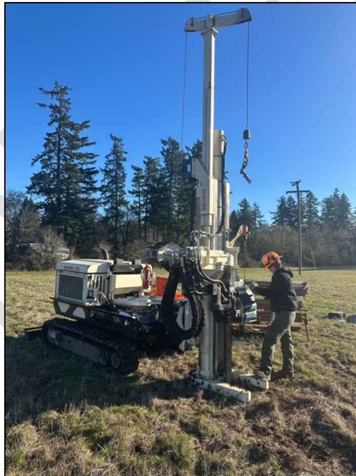
Figure 13 – Oregon State University (OSU) graduate student Gabby Ridenour operates a Geoprobe model 7822 DT coring rig to collect stratigraphic samples (Photo provided by Loren Davis).
