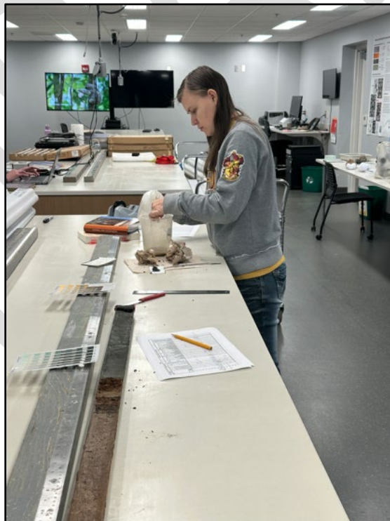
Figure 15 - Describing and recording soil and sediment data from a split Geoprobe core (Photo provided by Loren Davis).
