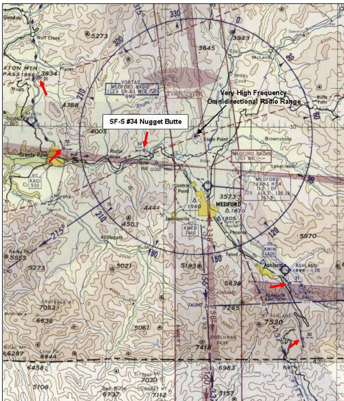
Figure 8. Detail of September 1960 Klamath Falls Sectional Aeronautical Chart (last sectional to show San Francisco-Seattle Airway Beacon #34 Nugget Butte) Red arrows point to the five remaining airway beacons in Jackson and Josephine Counties.
