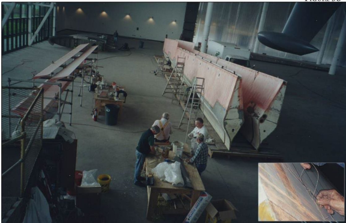
H-4 HERCULES -AILERONS RESTORED WITH NEW FABRIC SEWN ON BY HAND, 2001.
