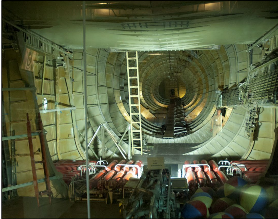
THE H-4 HERCULES CARGO DECK, LOOKING AFT FROM THE VIEWING CUBE TOWARD THE SEAPLANE'S TAIL. THE WINGS COME TOGETHER AT TOP OF THE IMAGE, ACCESSIBLE BY THE LADDER AT THE CENTER. THE RESTORATION CREW DISCOVERED THE BEACH BALLS (LOWER RIGHT) IN THE PONTOONS. NOTE THE RED CO 2 CANISTERS, WHICH ARE PART OF THE FIRE SUPPRESSION SYSTEM.
