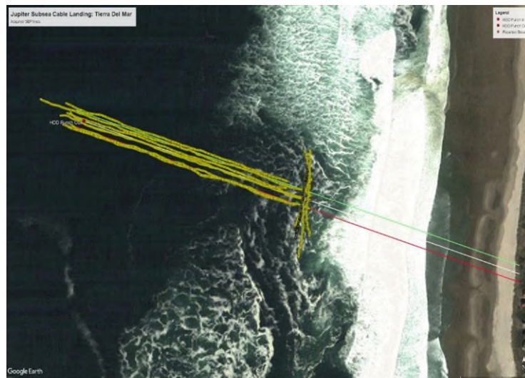
Figure 3..... Sub Bottom Profile Coverage acquired along the horizontal directional drill path.
