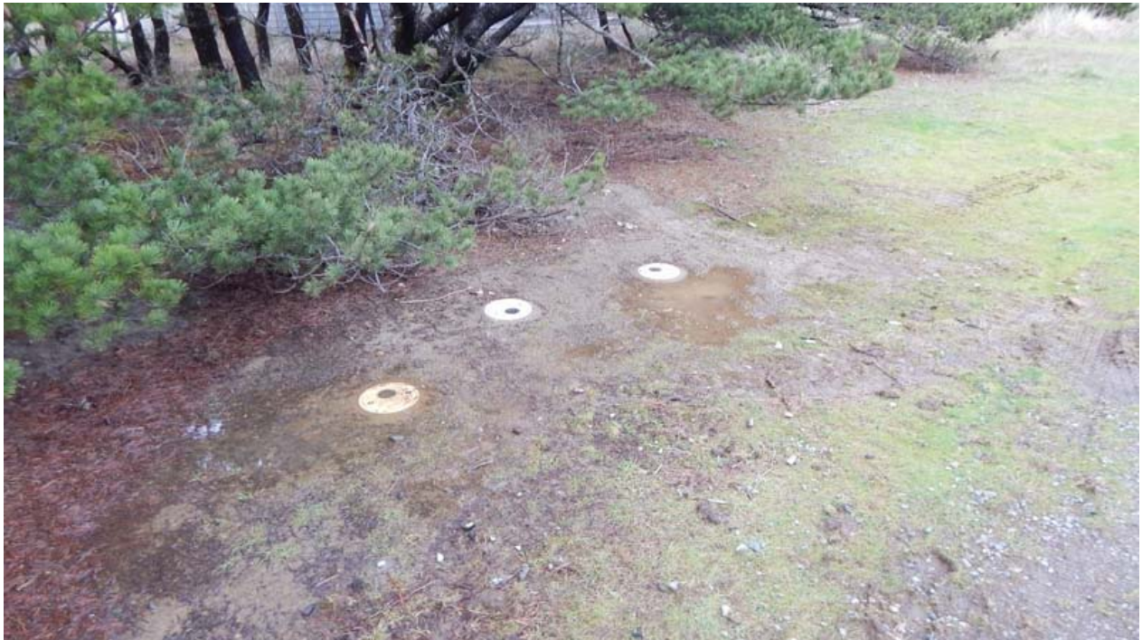
PGG-3 wells on Pollock Ave at 17:09 on March 2, 2018. Water has infiltrated and wells are now accessible.
