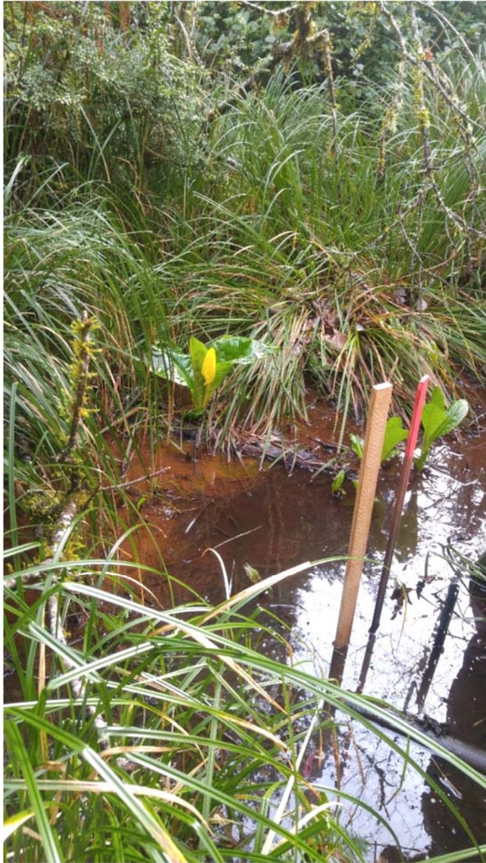
Marsh Stake #13 location east of Sand Lake Road. Note metal stake used for water level measurements and orange bacterial mats consistent with groundwater discharge to the marsh area.
