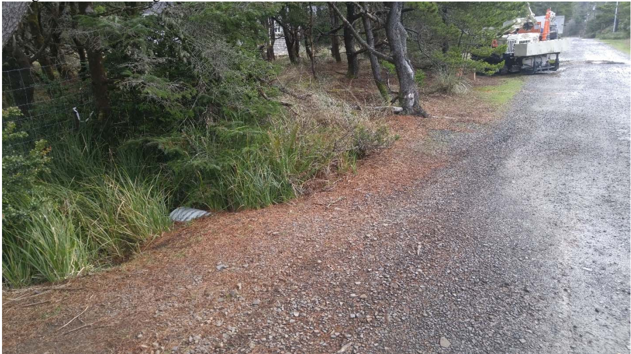
Drilling at location PGG-3 on Pollock Ave in background. Culvert for ditch running parallel to the fore-dune in foreground. A metal stake was set in the sedges to measure water levels when water is present. Water was only observed once in this ditch on March 1, 2018 during this study. Note that this ditch is different than the ditch paralleling Sand lake Road, which is located to the east.
