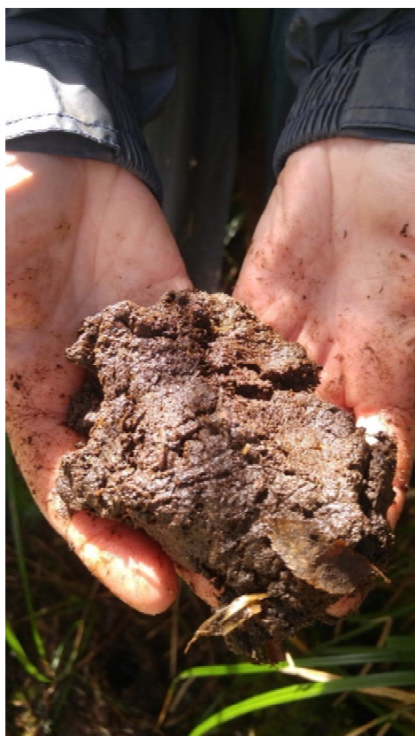
Example of soils observed in hand auger locations north of Roma Avenue. Soils consisted of fine sand with organics. No low-permeability skin was observed and hand auger boring filled with water quickly.
