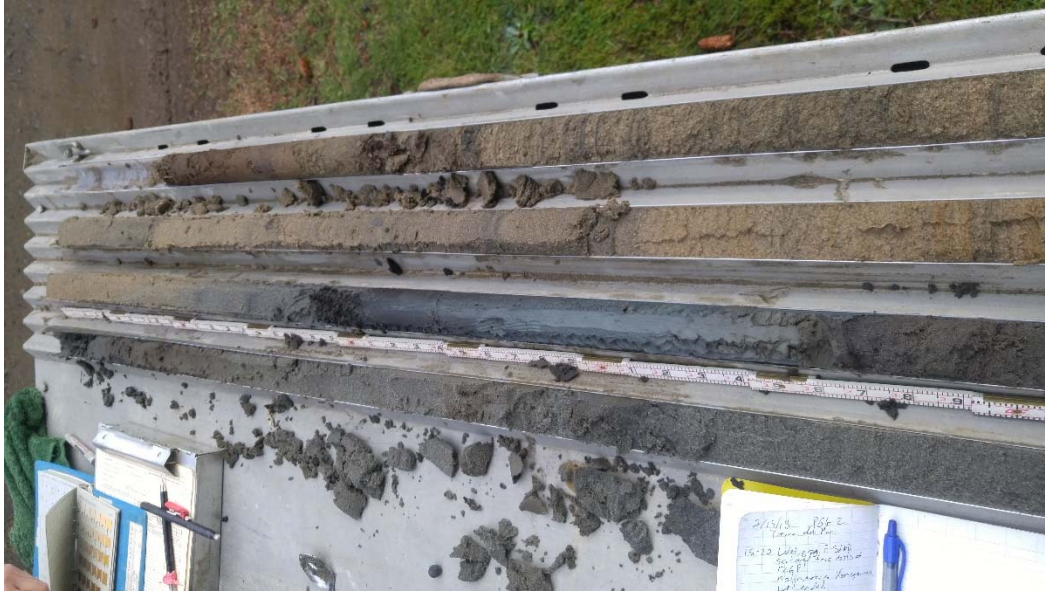
Soil cores at PGG-1. Arranged in 5-foot cores, top is shallowest core with top (up) on the right.
