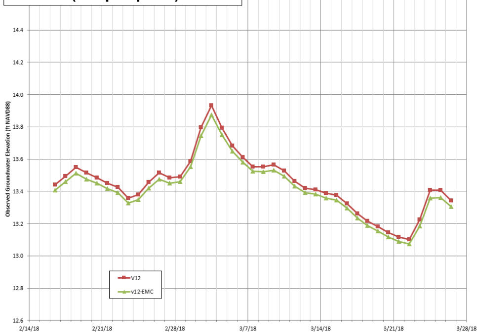
Figure I-4 Transient Calibration Comparison for Well PGG-2 Using the EMC Model
