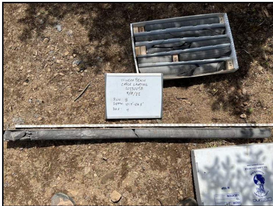
PHOTO 20: BORING B-1, CORE RUN 8: 101.5 FT - 106.5 FT
