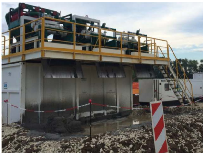
Figure 3: Example of a Drilling Fluid Mixing & Recycling Unit
