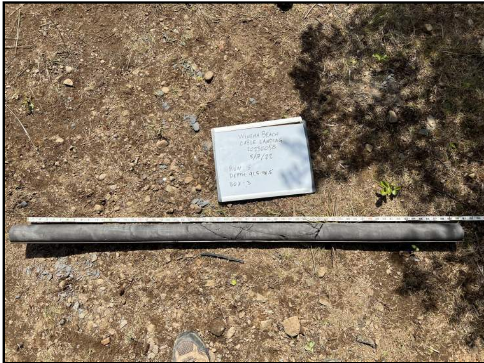
PHOTO 18: BORING B-1, CORE RUN 6: 91.5 FT - 96.5 FT
