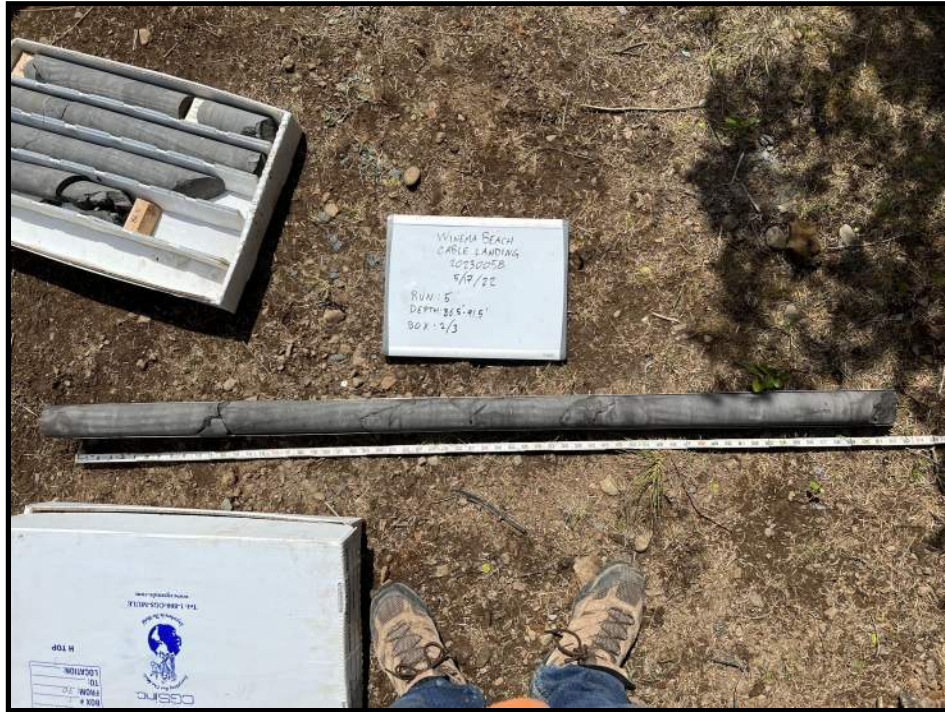
PHOTO 17: BORING B-1, CORE RUN 5: 86.5 FT -91.5 FT
