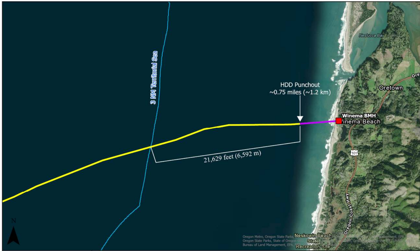
Fig. No. 3 Offshore Extent of Horizontal Directional Drill Cloverdale, Oregon Bifrost Submarine Cable
