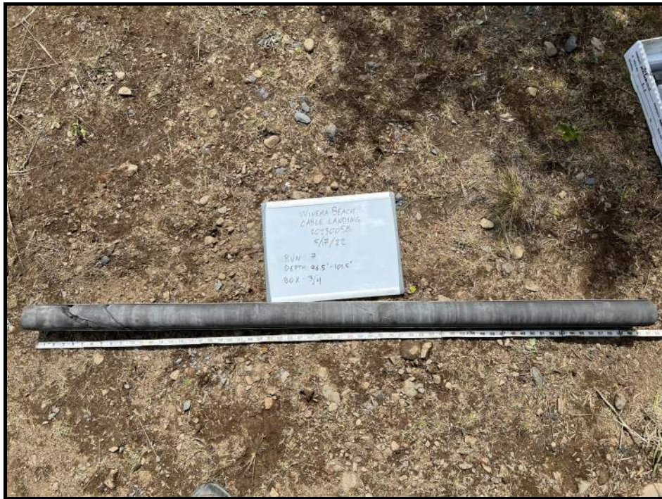
PHOTO 19: BORING B-1, CORE RUN 7: 96.5 FT - 101.5 FT
