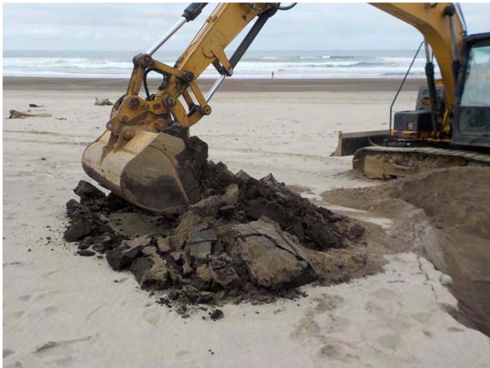
Photo 16 – View of the organic-rich silty soil spoils encountered in some of the test pits (From 02/24/2022).
