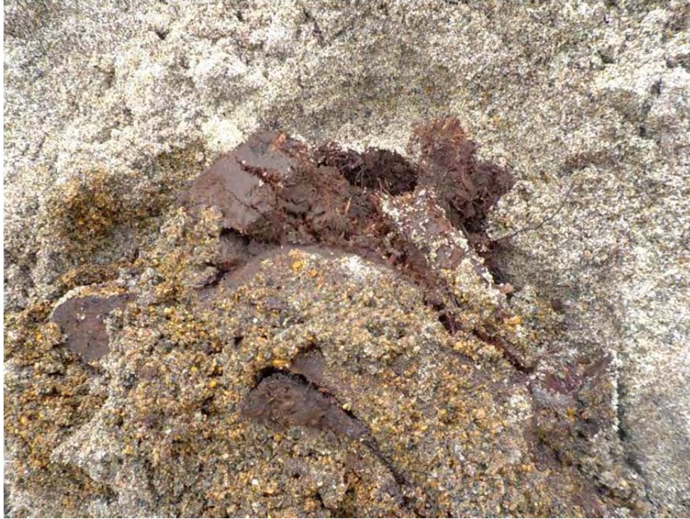
Photo 15 – Close-up view of the coarse sand and organic-rich silt and peat encountered in some of the test pits (From 02/24/2022).
