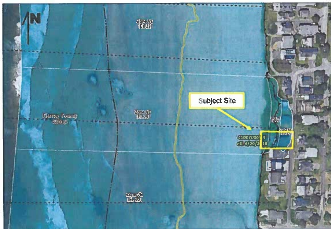
Figure 5: FEMA mapping showing the flood hazard layer in the project vicinity.
