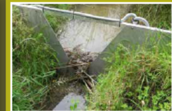
One of the more unusual challenges of working within a beaver enclosure is that water trickling through v-notch weirs triggers this instinctive behaviour by the beavers.
