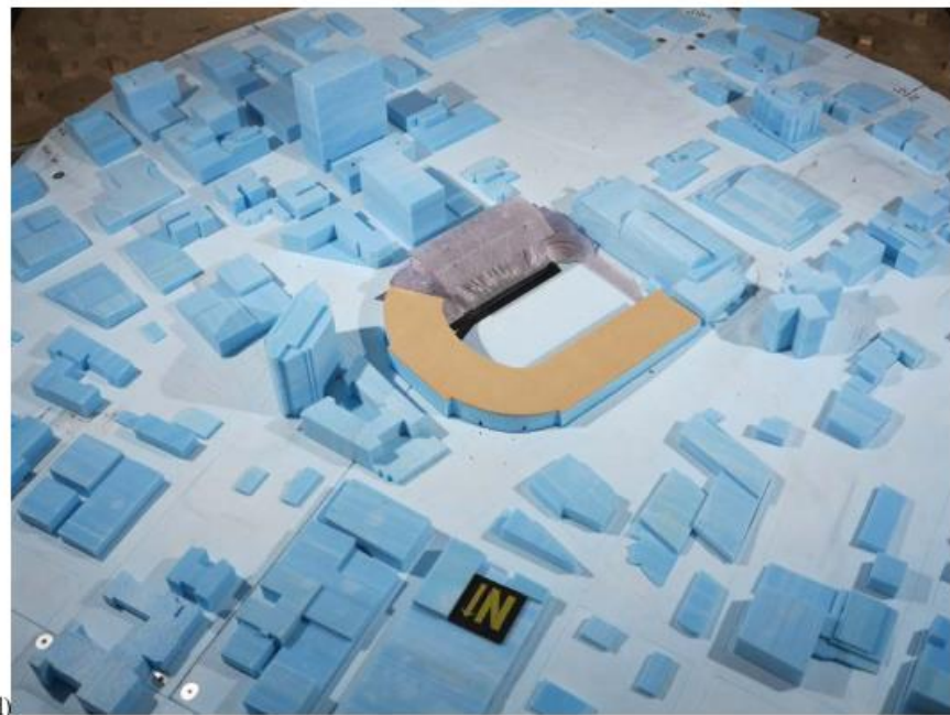
Figure 1. Photographs of the completed model in the wind tunnel: (c); (d) Overhead views of the model.
