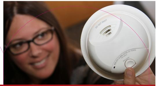
Smoke Alarms can be silenced by pushing the test button to quiet a nuisance alarm for up to 15 seconds.
