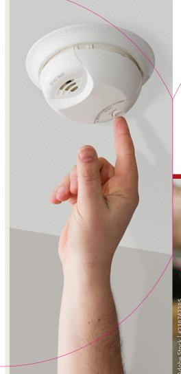
Smoke Alarms make a short chirping sound when their batteries are low, and three long beeps when there is smoke in the air.
