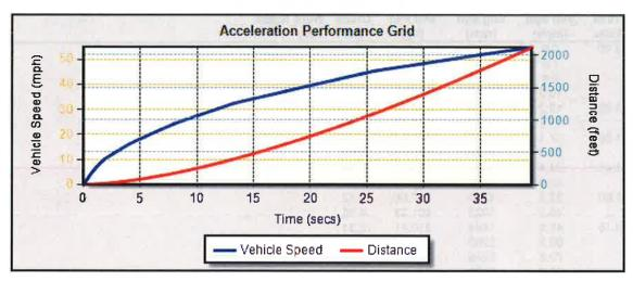
Acceleration Performance: TIME TO ACCELERATE ON A GRADE TO 55.0 (MPH) IS 39,57 (SECS)
