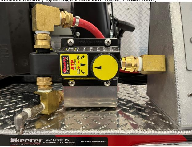
STEP 2: Open all discharges that were used with foam until the water is completely free of foam concentrate. (If you do not know if a discharge was used with foam, you should clean it out to verify)
