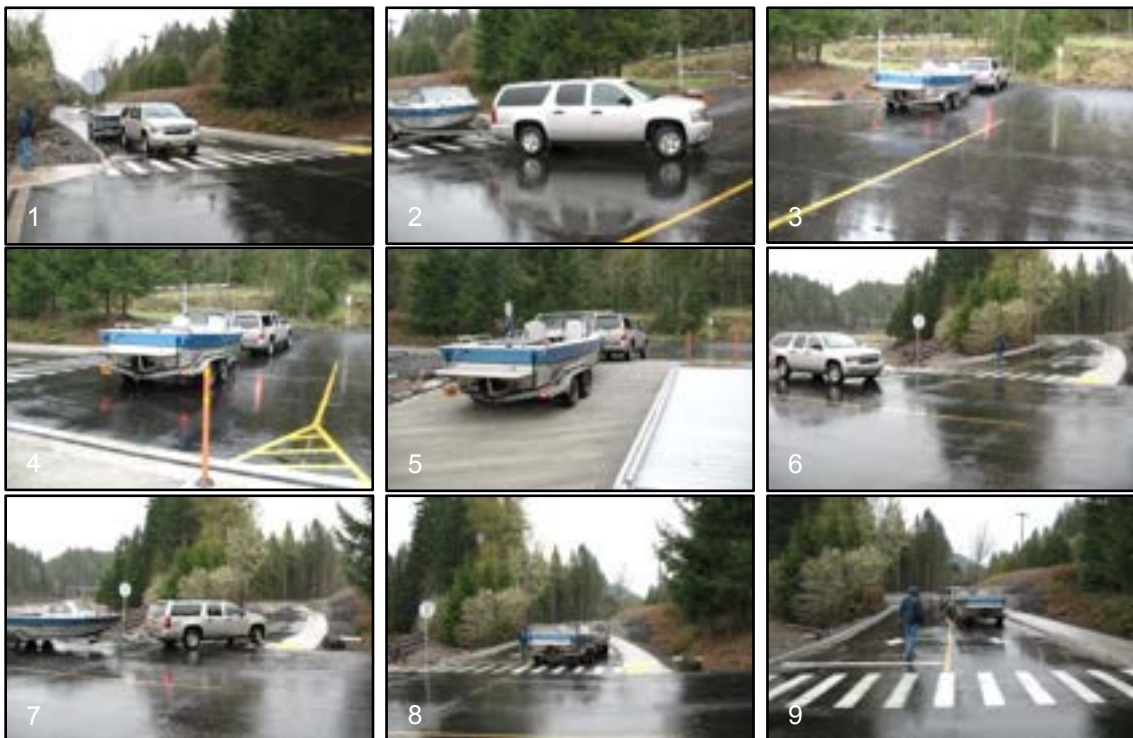
Photo 9-10 Photo series showing the maneuver area approach, alignment, backing, and departure
