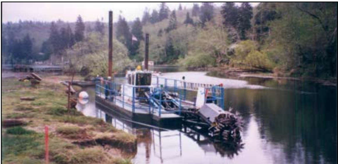
Photo 2-3 Suction dredging barge
