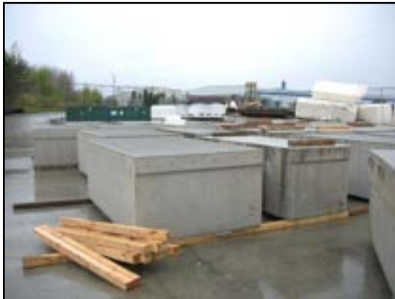
Photo 5-7 Individual concrete float sections
