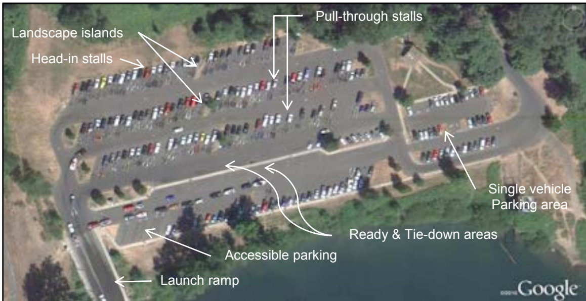
Photo 9-12 Aerial photo of a parking facility showing one-way traffic grid pattern and separation of boat trailer and single vehicle parking areas. Additional single vehicle stalls are incorporated at ends of landscape islands. This facility uses pull-through stalls to the maximum extent possible and head-in stalls along the perimeter.
