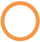
A circle of international orange with white center shall be used to indicate water zone within which a control or restriction is imposed upon operation of vessels and/or use of the zoned area. The nature of the control shall be indicated by words, numerals, or well-known abbreviations in black letters inside the circular shape, or above and/or below it.
