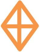
A diamond shape of international orange with a cross of the same color within it against a white center shall be used to indicate a water zone where vessels may not enter. Any words or well-known abbreviations must be in black letters above and/or below the shape on white background.
