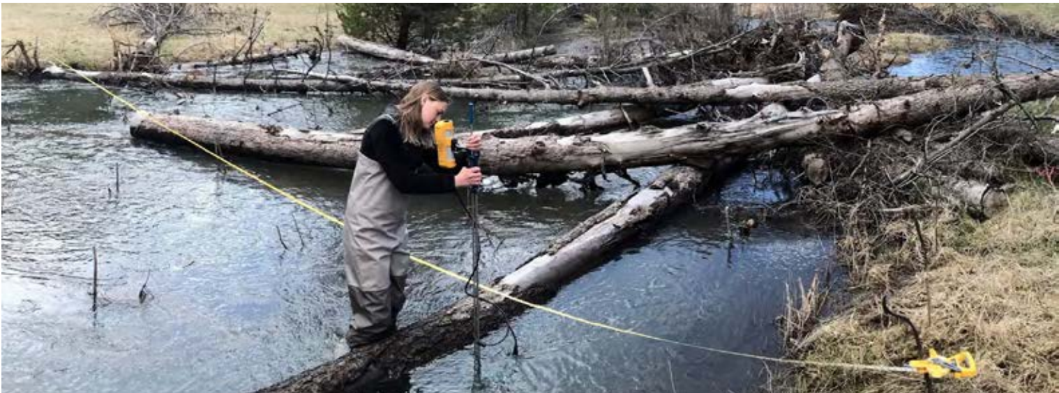
Grande Ronde Model Watershed staff measure streamflow on Limber Jim Creek. Monitoring investigates how streamflow timing and quantity may change as a result of large wood additions aimed at reconnecting the floodplain.
