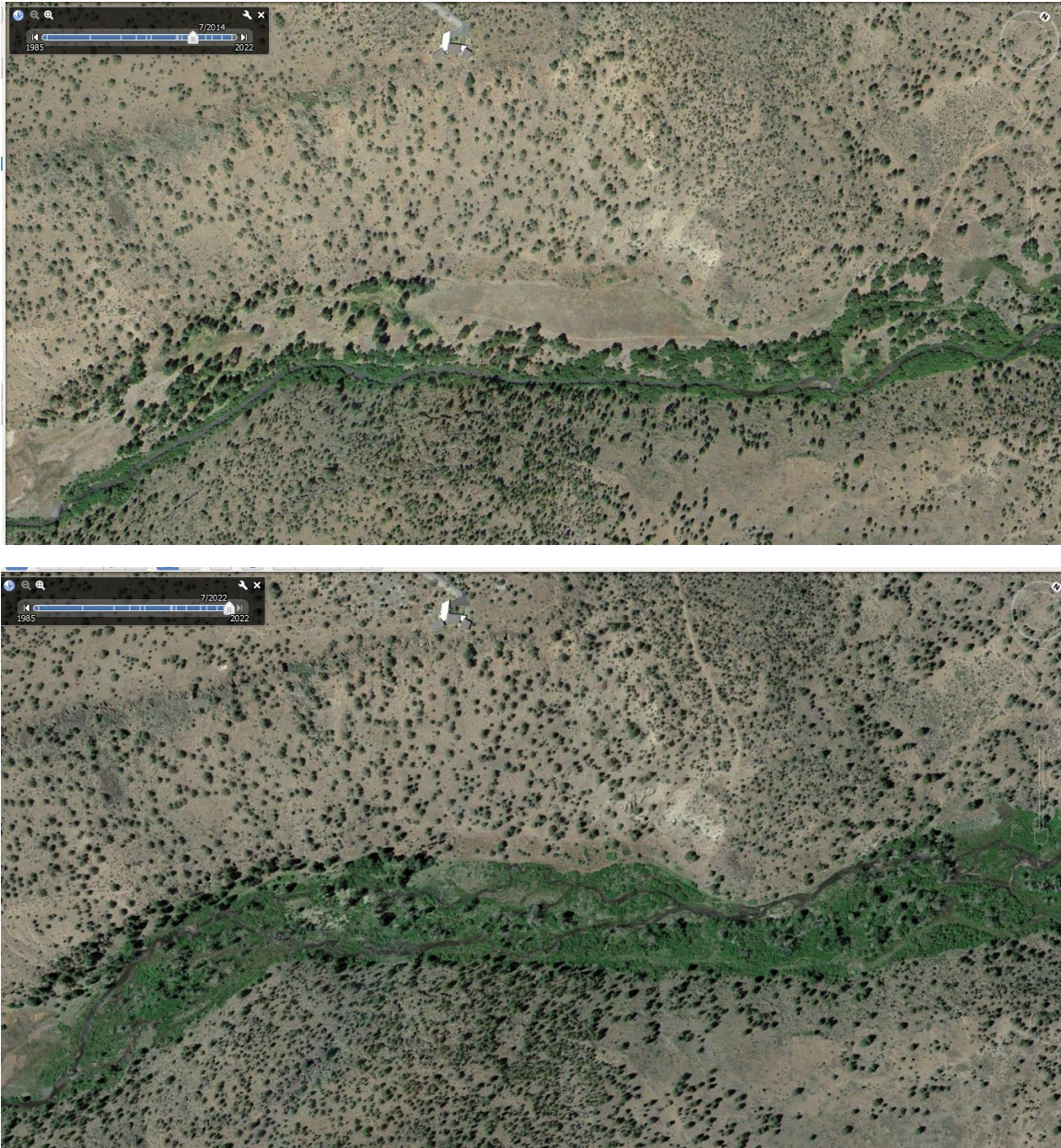
Figure 22. Visually observable differences in vegetation greenness and density in Whychus Canyon Phase 1 pre-restoration in July 2014 (top) and post-restoration in July 2022 (bottom) suggest NDVI or NDWI might be good candidate methods for classifying riparian vegetation in restoration reaches.
