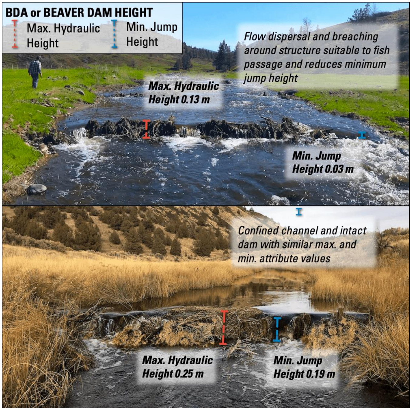
FIGURE 13. EXAMPLES OF BEAVER DAM OR DAM ANALOG MEASUREMENTS OF MAXIMUM HYDRAULIC HEIGHT AND MINIMUM JUMP HEIGHT WITHIN TWO DIFFERENT CHANNEL AND STRUCTURE SETTINGS.
