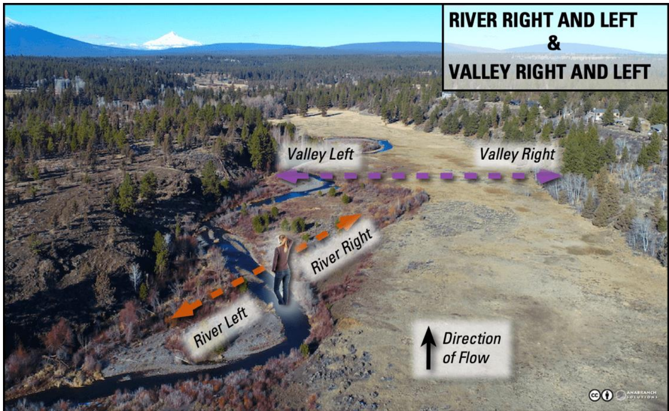
FIGURE 6. DEMONSTRATION OF DIFFERENCE BETWEEN RIVER LEFT AND RIGHT, WHICH WILL FOLLOW THE PLANFORM OF THE CHANNEL, AND VALLEY LEFT AND RIGHT, WHICH WILL FOLLOW THE PLANFORM OF THE CONFINING VALLEY MARGINS.
