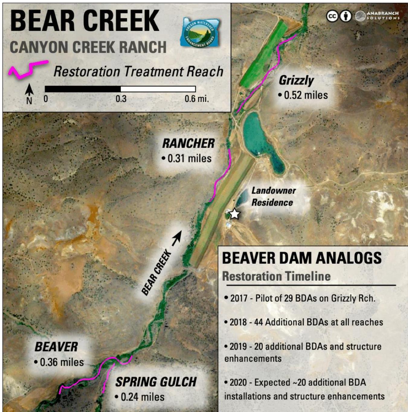
FIGURE 3. EXAMPLE OF A PROCESS-BASED RESTORATION PROJECT DESIGN CONSISTING OF MULTIPLE TREATMENT REACHES DELINEATED ACCORDING TO VALLEY AND FLOODPLAIN CHARACTERISTICS THAT DETERMINED RESTORATION POTENTIAL AND OBJECTIVES. EACH REACH ALSO CONTAINS SEVERAL STRUCTURE COMPLEXES PROJECT IMPLEMENTATION CONSISTED OF AN INITIAL PILOT THAT WAS FOLLOWED BY 3 ADDITIONAL PHASES OF STRUCTURE ADDITIONS, MODIFICATIONS, AND ENHANCEMENTS IMPLEMENTED ANNUALLY.
