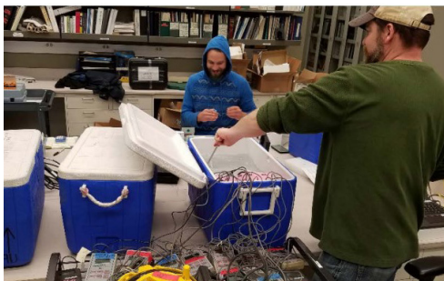
DEQ staff checking volunteer monitoring partners field instruments against National Institute of Standards and Technology (NIST) certified standards. Photo from DEQ Water Quality Monitoring Strategy 2020 .
