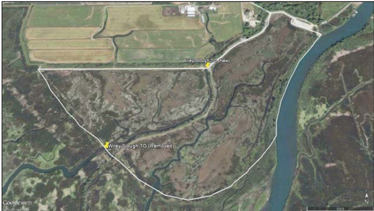
Aerial Images: Wiley Slough tide gate relocation and tidal reconnection (8/3/2016).
