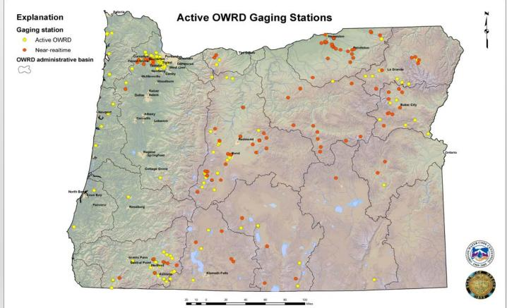
The Water Resources Department operates more than 200 stream and reservoir gages throughout the state. About 110 of these gages are operated as near real-time. These gages transmit stream data once an hour. This data is received and downloaded to the Department's database where it is processed and the streamflow information is updated on the web page every hour. In addition, information from another 225 gages operated by the USGS and other agencies is also shared on the Department's website.
