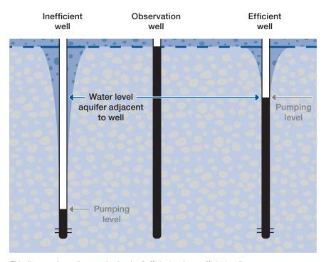
This diagram shows the pumping levels of efficient and non-efficient wells.
