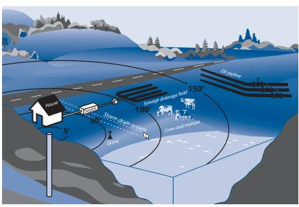
This diagram represents common contamination sources and required setbacks for domestic wells.
