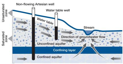
This diagram shows a typical aquifer system. Common definitions of groundwater and well terms are included in the back of this booklet.
