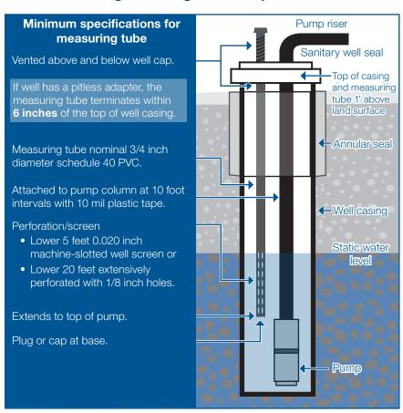
This diagram details the minimum standards for a dedicated measuring tube. The dedicated measuring tube shall not be reduced in size over the length of the pipe and shall remain free from wires and other obstruction.
