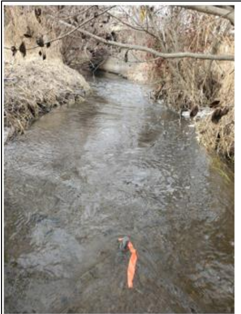
A temperature rod deployed in a stream with orange flagging to spot during retrieval.
