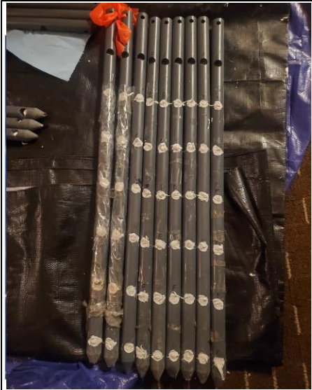
Temperature rods being prepped before deployment, white silicon seals the temperature sensors from water.
