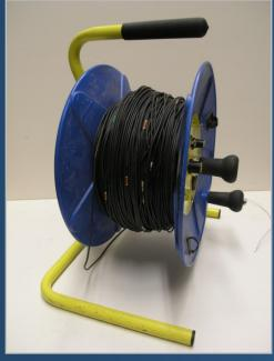
Use in wells with narrow access, an installed pump, or possible obstructions Flat E-Tape
