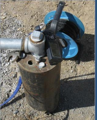
Remove Column Plug to Access Inside Column
