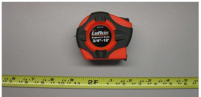
Co-axial e-tape measurements require the additional use of an engineer's tape measure to obtain measurements to the nearest 1/100<sup>th</sup> foot. The engineer's tape measure is marked in feet, 1/10<sup>th</sup> foot, 1/100<sup>th</sup> foot, and inches.
