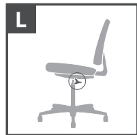
L. Tilt lock — Locks out tilt function when chair is in upright position.
