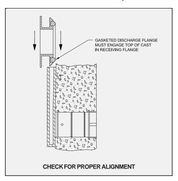
position. If allowed to tilt, the system could rub the edge of the concrete opening and be damaged. **NOTE:** Use the viewing port to be sure proper alignment and engagement of the outlet connection takes place. The discharge flange must engage the top of the cast-in-place receiving flange.
