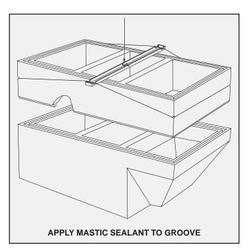
The top casting may now be set. Remove all debris from the bottom of the casting along the tongue sealing section. Do not reach or get under any portion of the casting. Carefully position the top and lower one corner into the groove. Align the sides of the casting and lower the top into position. Before proceeding with Bio-Static sludge return assembly and installation, recheck the tank for level from side to side and end to end.
