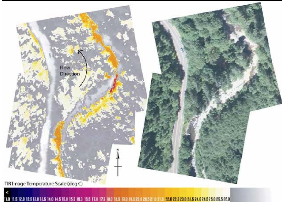
Figure 13.6 TIR/color video image pair showing the location of a spring (16.6°C) on the right bank of Sharps Creek (20.4°C) at RM 8.2 (frames: shar0540-0544). July 21, 2002.
